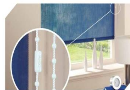
Chain break connector will part under any undue load but after inspection can be clipped back together again
